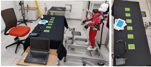
Figure 1: Game room setup with a deck of six cards with blue back, six green marks on the table and the Tobii Pro Glasses 2 eyetracker.
